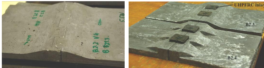
Figure 6: Advanced bending joint design B2.2 with thickened dovetail anchor (left), B2.3 doubled joint and B2.4 shape optimized joint with UHPFRC inlay (right)
